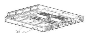
1-2 Non-hot plug SATA hard drive bays - Using quick release carrier
