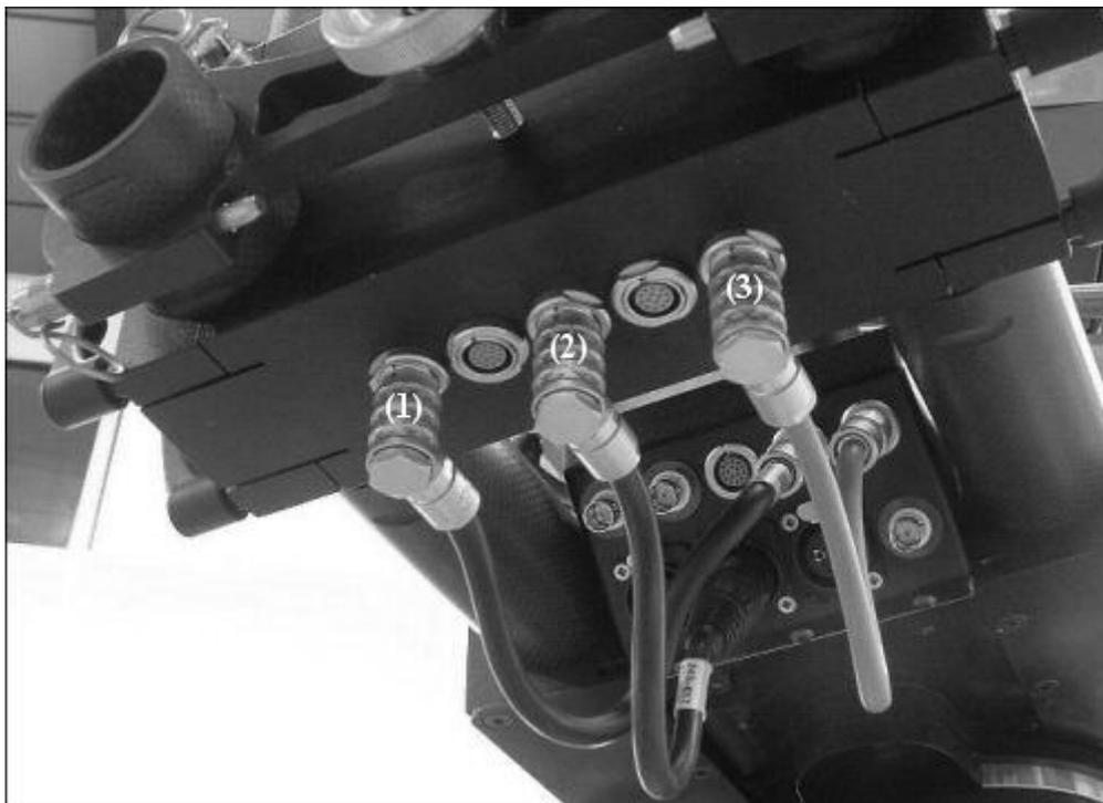
*Figure 35. Ulti-Head Slip-Ring lower panel and Ulti-Head Elbow lower panel with (Flair) connections*
