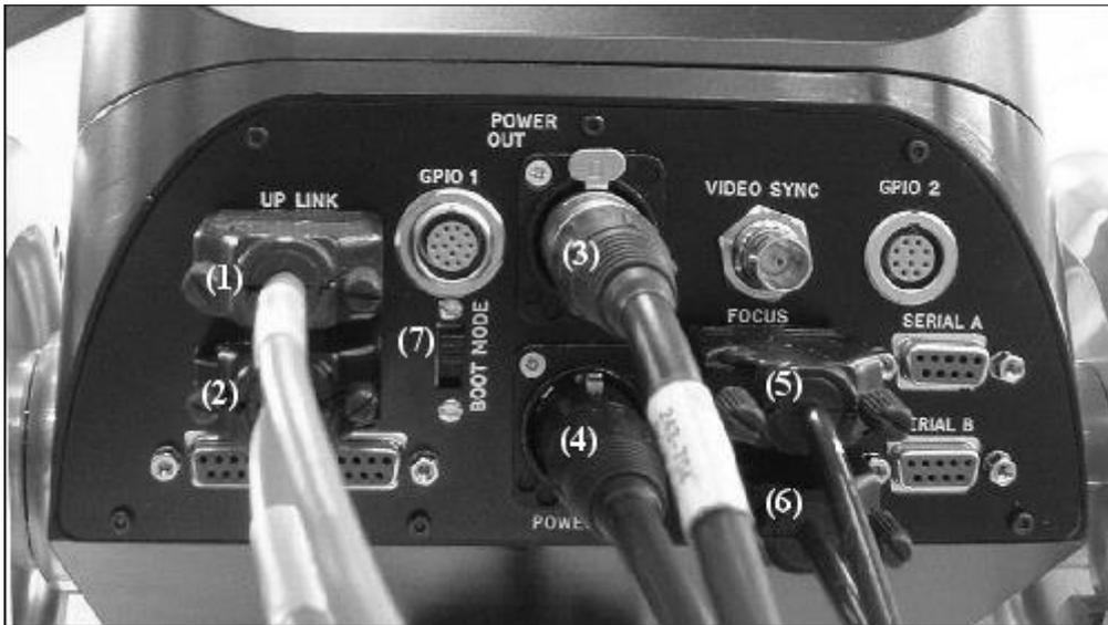
Figure 33. MSA-20 rear panel with (Flair) connections
