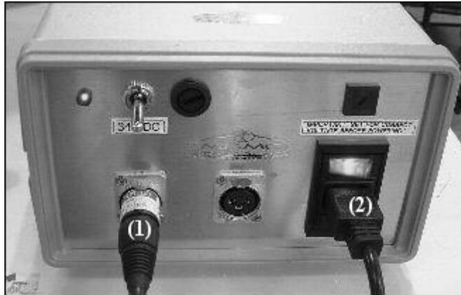
Figure 23. Power Supply Unit with connections
