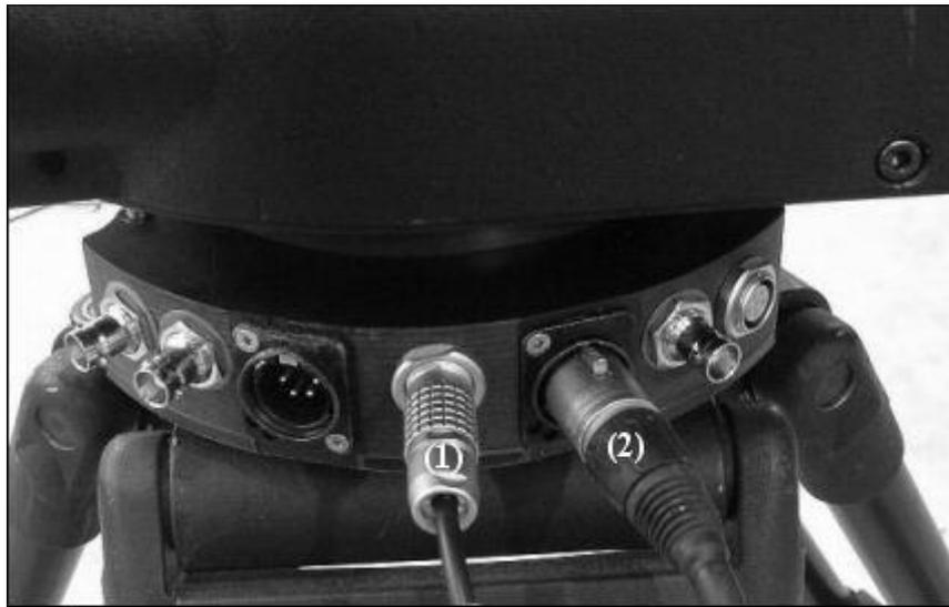
*Figure 25. Ulti-Head Slip-Ring side panel with (Standalone) connections*
