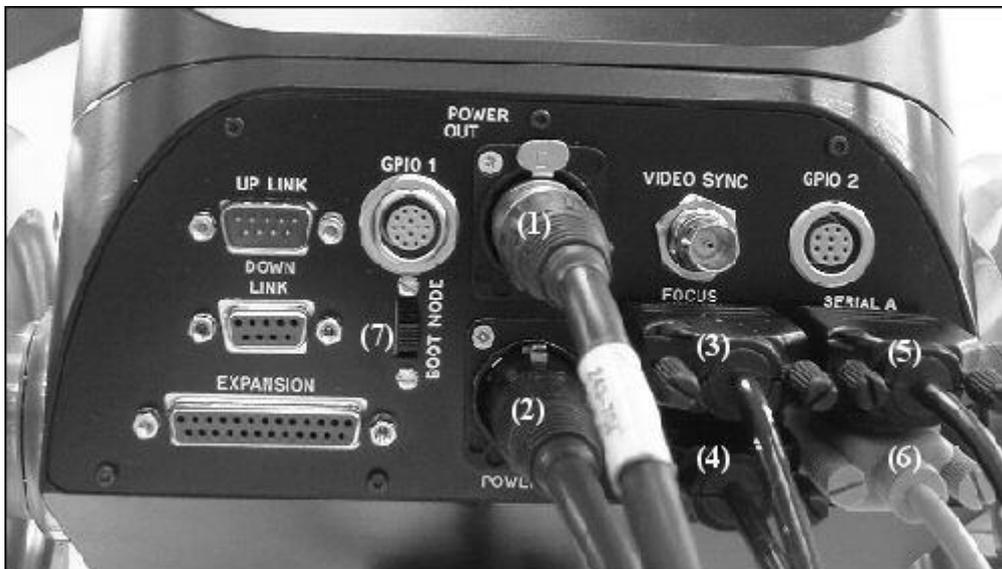
Figure 24. MSA-20 rear panel with (Standalone) connections
